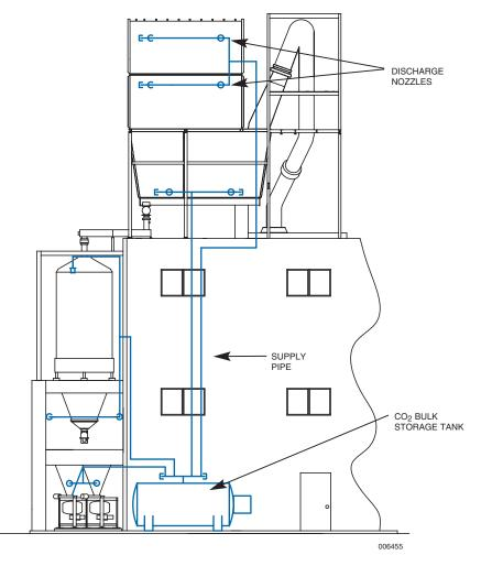
**NOTE:** This drawing represents an elevation view of a typical low pressure CO<sub>2</sub> system protecting a dust collector. For clarity, the detection system is not shown.
