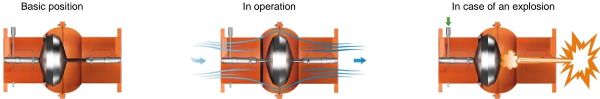
/ In case of an explosion, the pressure wave pushes the closing device (without external energy supply) against the valve gasket.
